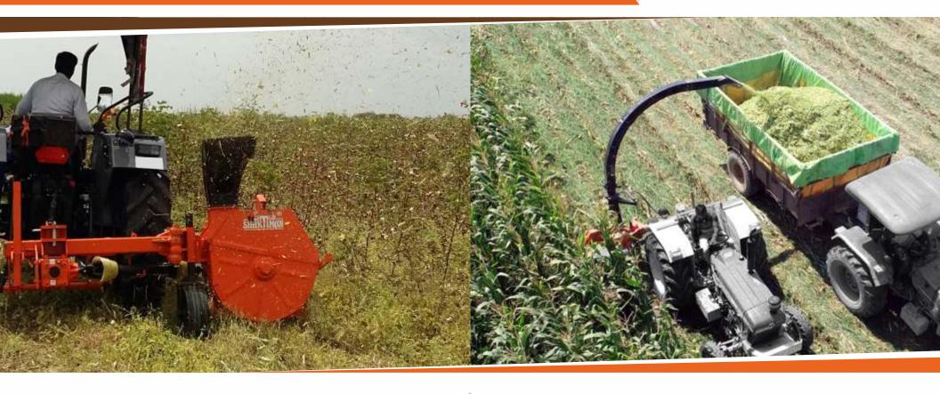
**SHAKTIMAN** Mobile Shredder is a tractor operated agricultural equipment for cutting and shredding crop stalks to clear the field faster for next crop. Suitable for row crops like cotton, castor, maize, chilli and other similar crops. Machine can be operated by any 40 and above hp tractor with dual clutch, attached to 3 point linkage and powered by PTO with 540/1000 rpm through driveshaft.
