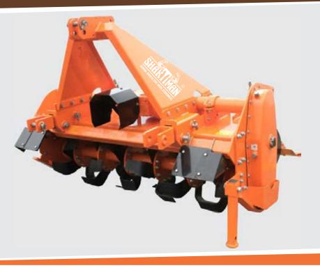
SHAKTIMAN offers a wide range of Rotary tillers to customer to select the right product for their tillage need depended on the type of soil, type of crop and depth required.
