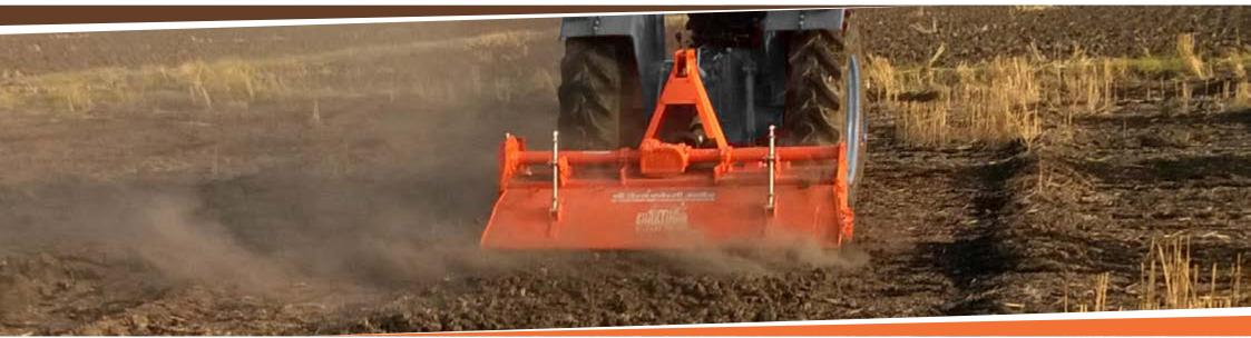
**SHAKTIMAN** Regular Plus Series Rotary Tillers, with simple construction but strong design are appropriate for dry land application in hard soil and wet land cultivation in light soil and deep puddling. Available in wide range of working widths to suit 25 to 60 HP tractors.
