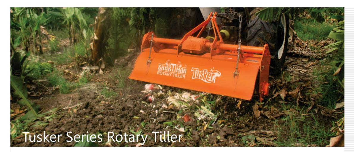
Tusker Series Rotary Tiller is specially designed for crushing of banana stem and pulverizes it within soil in a single pass. It is suitable for slashing thick and fibrous residue of crops such as banana, papaya, sugarcane etc. Pulverization of the crop residue, increases soil fertility & permeability. It also increases aeration & water holding capacity of the soil. It is ideal for sandy & sandy loam soils.
