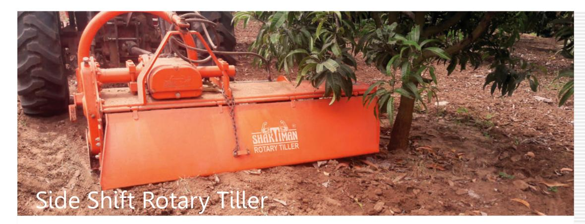
**SHAKTIMAN** Side Shift Rotary Tiller is particularly designed for the purpose of delivering an impactful performance in central as well as offset position. This feature allows operating the tiller in areas where tractors have limited access due to their size and also in areas with low-hanging branches of trees. The side shift system of the tiller is based on a hydraulic cylinder. It can be
