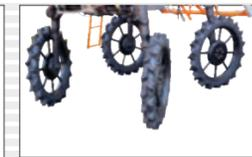
All-wheel drive with smaller turning radius of 2.9 mtr
