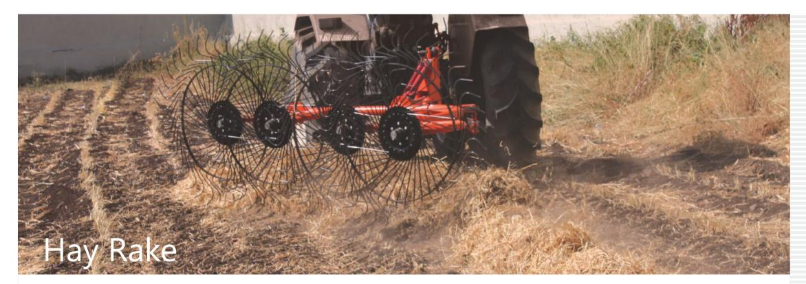
**SHAKTIMAN** Hay Rake is designed to move the mowed windrow across the soil surface or remaining crop stubble, creating a narrower windrow that will dry more rapidly.
